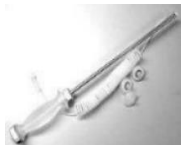
008-3015-200 Remote Teflon® sample draw kit for pump equipped multi-sensor instruments. Kit includes a stiff 10" (26 cm) aluminum sample probe with replaceable particulate and hydrophobic barrier filters, 3 hydrophobic barrier filters, 10' (3 m) self-coiling Teflon® tubing with Luer-style quick-connect fittings. (For use with PID equipped instruments)
